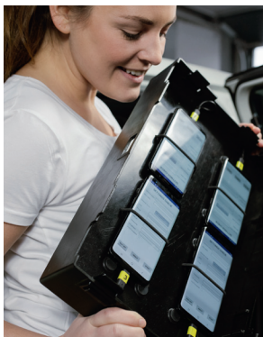
Each drive test vehicle carried eight smartphones for conducting the voice and data tests.
