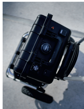
The walktest teams use trolleys in which powerful rechargeable batteries feed the test smartphones.
