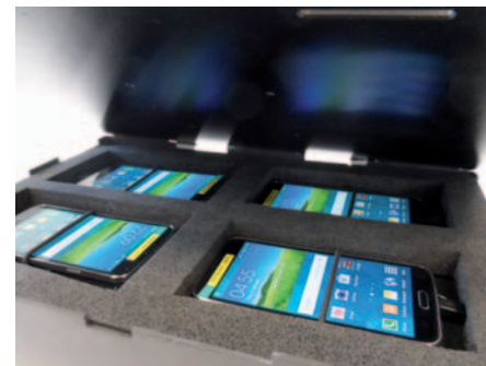
Up to three P3 Antenuatr-Boxes can be mounted into the back and side windows of each measuring car and up to four smartphones can be used to test up to four providers simultaneously.
