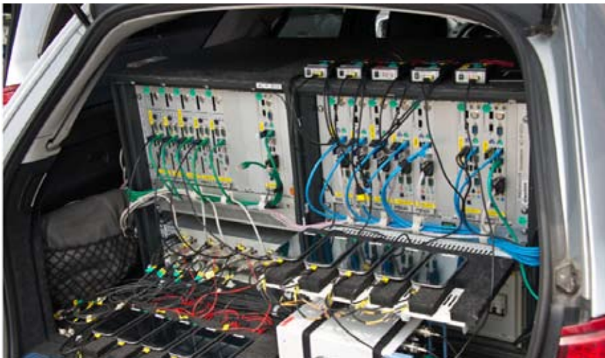
Measurement equipment of one of the two cars establishing the mobile to mobile calls.
