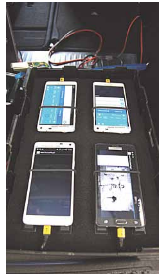
Four Samsung Galaxy Note 4 measured the data performance in German and Austrian networks.
