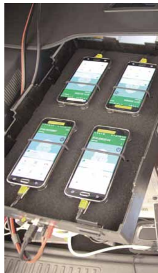
The voice tests and a part of the data tests were performed with Samsung Galaxy S7 smartphones.
