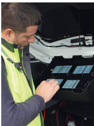
Each drivetest vehicle carried six Samsung Galaxy S8 smartphones.
