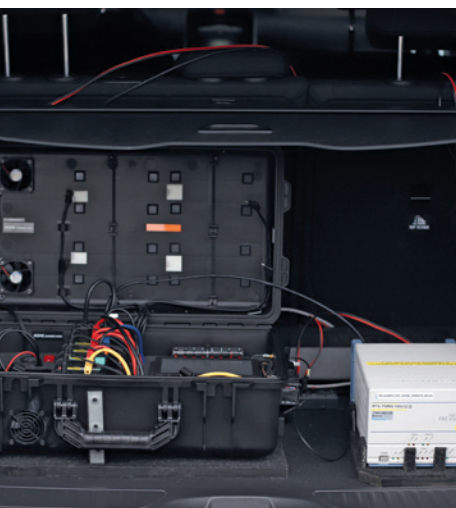
P3's proprietary control electronics manages the smartphones during the drivetests and collects all logged data.
