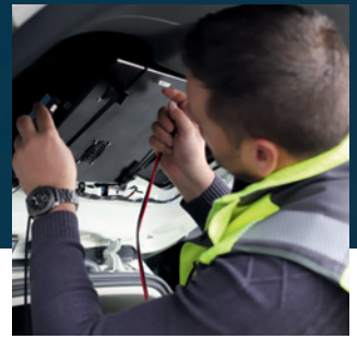
Boxes mounted to the rear and side windows of the cars contain the smartphones used for testing.
