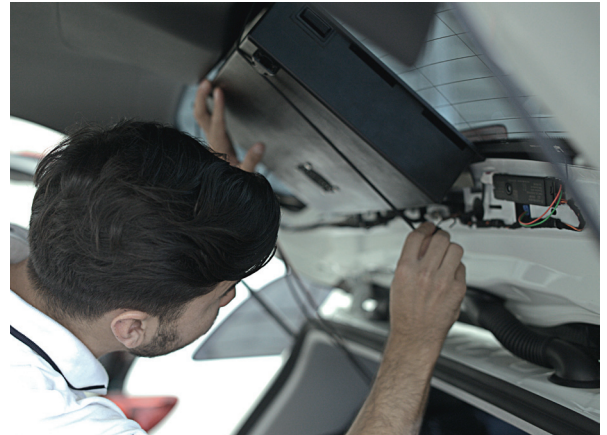
Three boxes were mounted into the back and into the side windows of each measurement car in order to support twelve smartphones per car.
