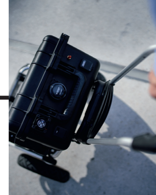
The walk test teams used trolleys or backpacks, in which strong batteries powered the test smartphones.
