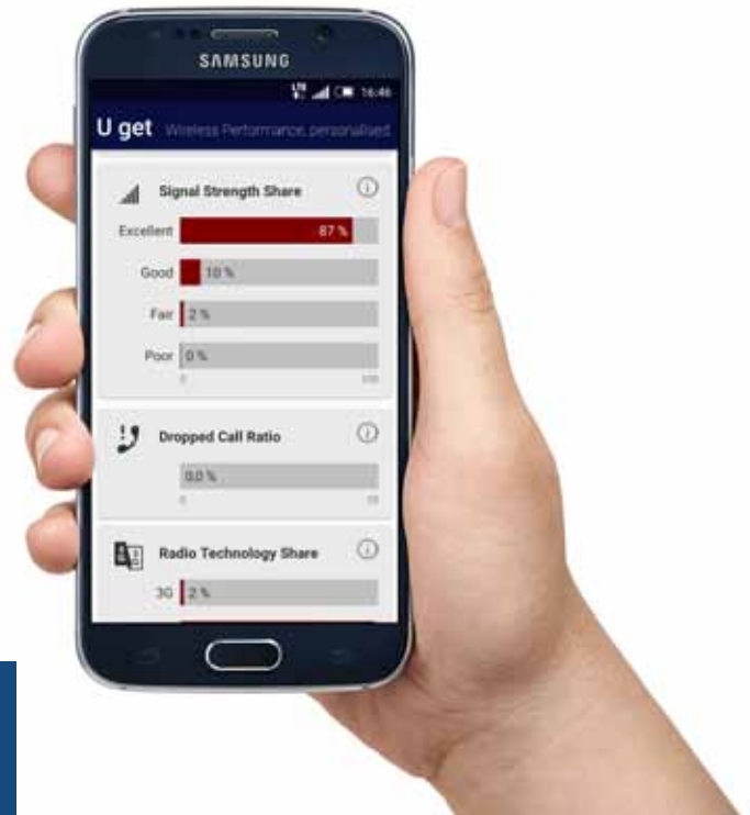
The collection of crowdsourced data is based on apps like “U get” (see below) and others, that constantly perform and report anonymised service availability measurements in the background.
