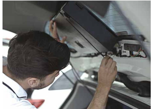
Three boxes were mounted into the back and side windows of each measuring car in order to support twelve smartphones per car.
