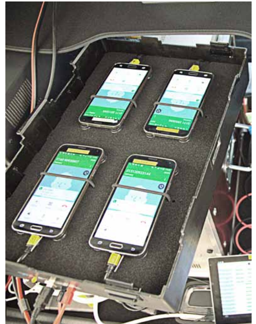
Each box was housing four smartphones which allowed the simultaneous testing of four mobile operators.
