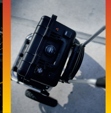
The walk test teams used trolleys or backpacks with powerful batteries to power the test smartphones.
