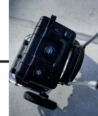
The walktest teams use trolleys or backpacks in which powerful rechargeable batteries feed the test smartphones.
