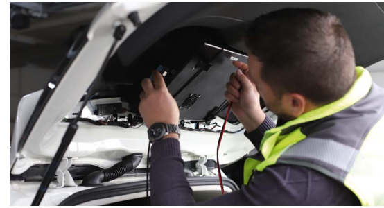
Two boxes were mounted into the rear and side windows of each measurement car in order to support eight smartphones per car.
