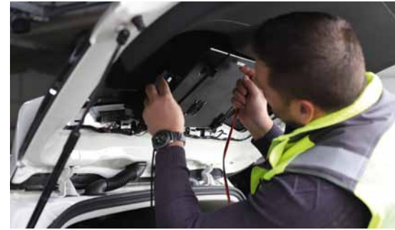
Two boxes were mounted into the rear and side windows of each measurement car in order to support eight smartphones per car.
