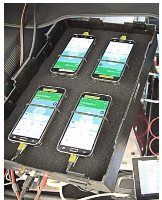
Each car carried four phones for the data tests and eight phones for the voice tests. They were housed in three special boxes, containing four smartphones each.
