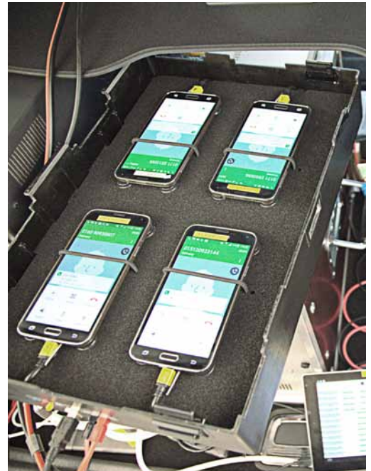
Each box housed four smartphones which allowed the simultaneous testing of four mobile operators.
