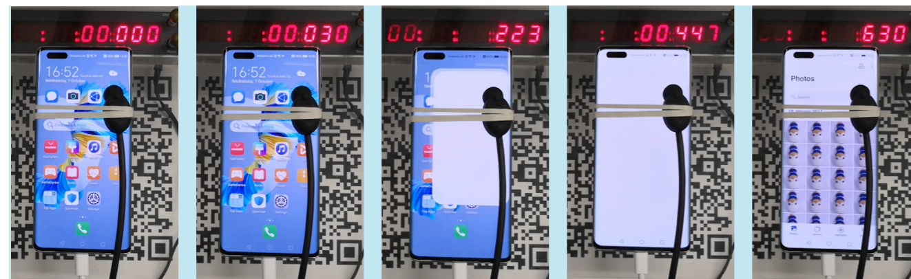
The analysis of the recorded video of an action allows the individual steps and the total time to be exactly timed. The picture shows the opening of the picture gallery with a sample photo. At the end of the action the total time is displayed on the stopwatch. Several repetitions guarantee high accuracy.
