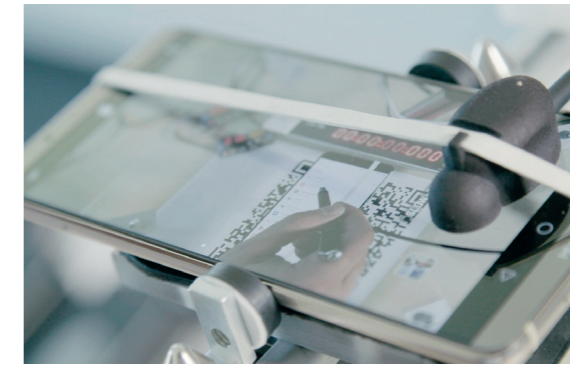
The virtual finger ensures a very accurate starting point of every action to be measured.
