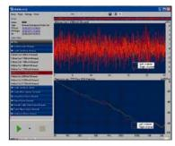
addition to these parameters, the Testlab measures defects such as noise and the echo disturbances that often occur in telephony.
