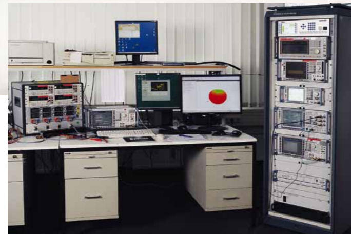
The endurance test site consists out of several high precision power supplies, PC controlable and readable system multimeters and Wideband Radio Communication Testers for GSM, UMTS and LTE.
