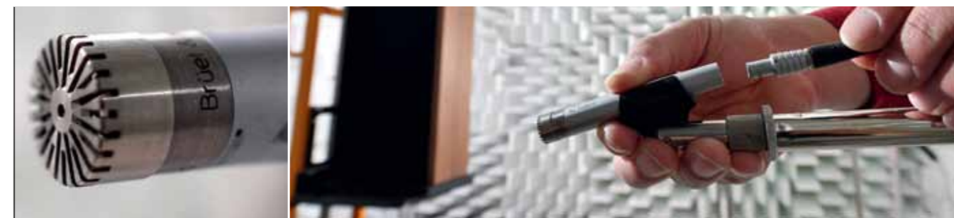
ONLY THE BEST: the microphone capsules B&K 4191 operate completely linearly from 3 hertz to 40 kilohertz, and from 20 to 162 dB (re 20 µPa).
