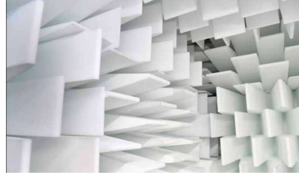
SOAKED: Absorber attenuate sound waves hitting the walls of the measurement chamber.
