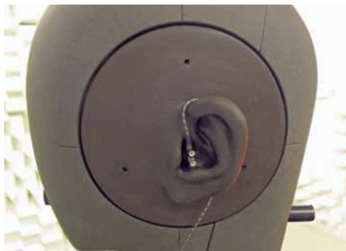
In-ear headphones must demonstrate their linearity on an HMS II dummy head of Herzogenrath-based Head Acoustics. The outer ear made of rubber (installed for the photo) is removed for the measurement.
