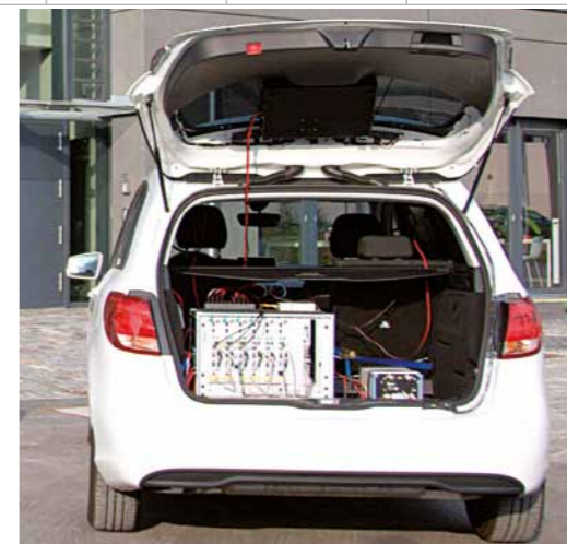
A computer array in each car was used to control twelve Samsung Smartphones for the measurements.
