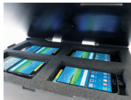
Three P3 Antenuatr-Boxes are mounted into the back and side windows of each measuring car and four smartphones are used to test four operators simultaneously.
